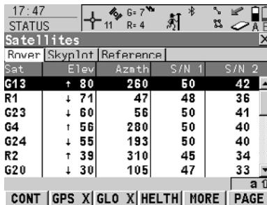
The screenshot shows a handheld device screen with a status bar at the top (17:47, STATUS, G=7, R=4) and a 'Satellites' window. The window has a title bar and a close button. Below the title bar is a table with columns: Rvr, SkypInt, Reference, Sat, Elev, Azimuth, S/N 1, S/N 2. The table contains data for satellites G13, R1, G23, G4, G24, R2, and G20. At the bottom of the window is a menu with buttons: CONT, GPS X, GLO X, HELTH, MORE, PAGE.
